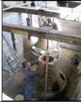
Fig 4 Building the bell mould at Villedieu les Poêles in Normandy
